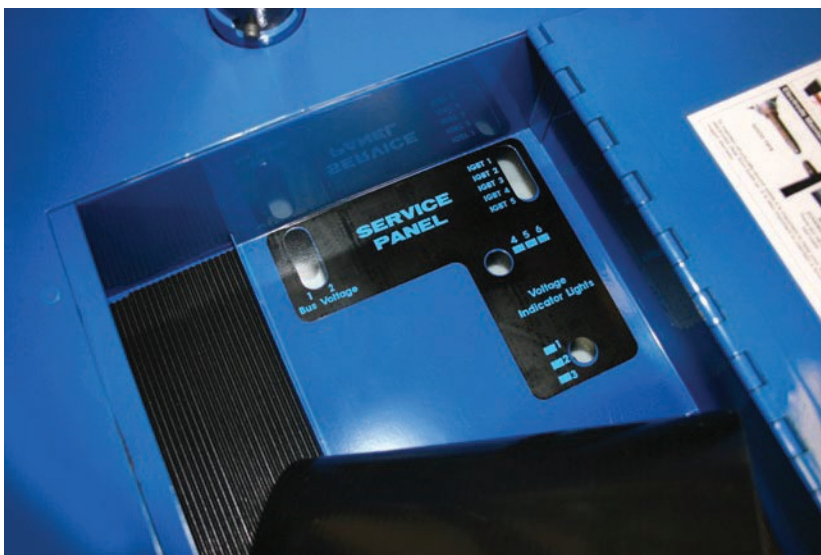
Service Panel Window – Control System Status Lamps
