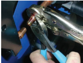
Figure 5.6b: Removing Welding Cap
