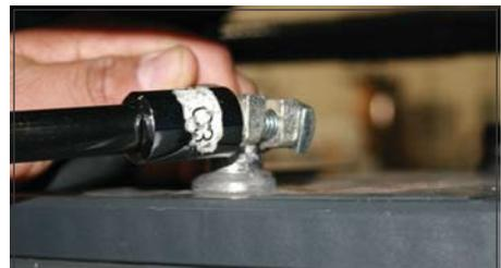
Place the leads (red on positive and black on negative) on the battery terminals and tighten with a 1/2" socket. Do not over tighten.
