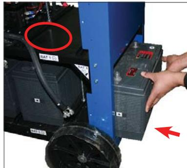
The rear lower battery has to be installed from the opening in the back of the welder.
