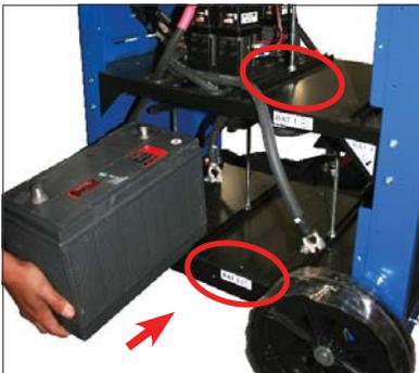
Insert batteries from the side, be sure to put check the labels (circled in the image) and set the batteries poles facing the correct direction.
