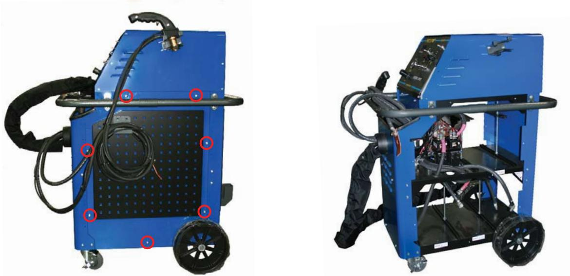
When you first receive your hybrid battery spot welder you will need to purchase 4 - 31P batteries at  $\geq 1000A$  that have pole style car battery terminals. Remove the 7 screws on both side panels and then remove the panels.
