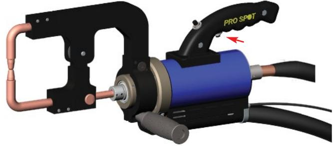
Push the lower switch to close electrodes and weld.
