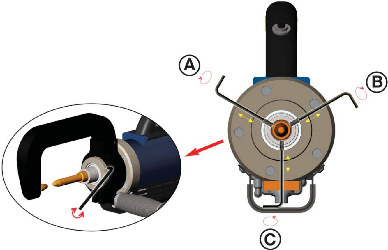
Figure 5.5 Electrode Alignment
