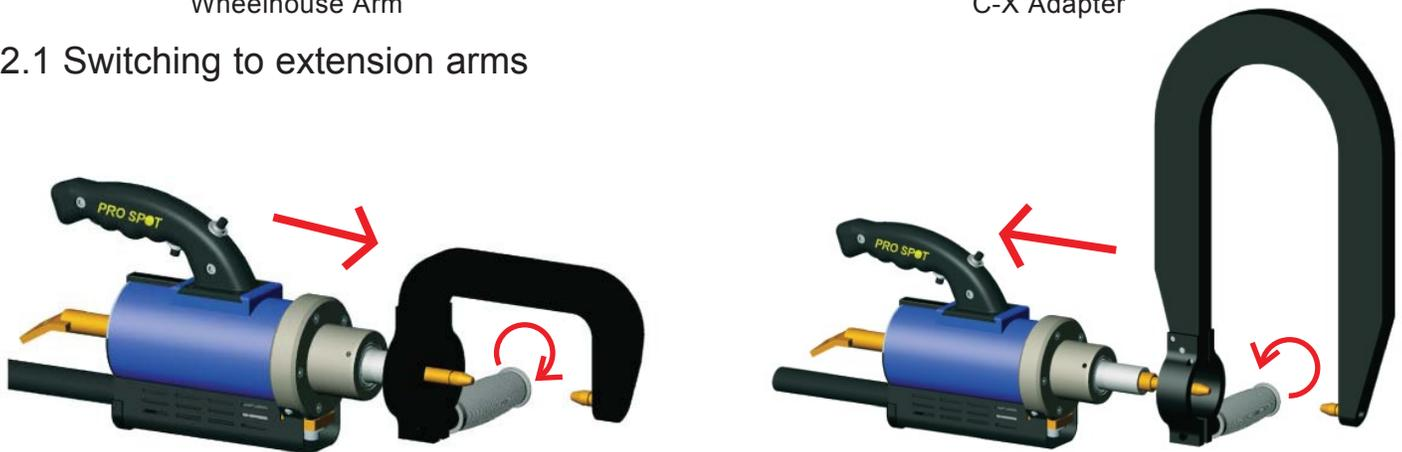
Loosen the handle and pull off the C-arm...
